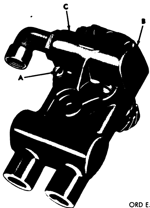
Figure 3-42. Removing or installing housing cover.
